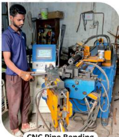
CNC Pipe Bending
