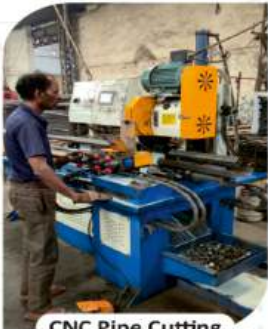
CNC Pipe Cutting
